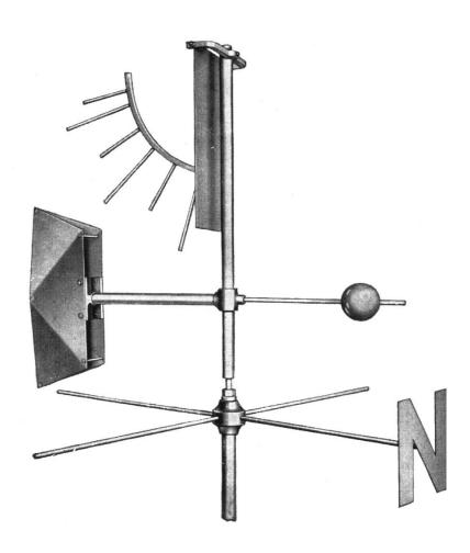
The Wind Vane No. 98 with Force Indicator Wild Type (Standard model of the German Meteorological Service) is of solid construction. A total height of 1.60 m facilitates accurate reading also from a considerable distance.
