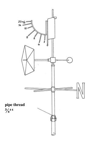
The N-mark fixed to the direction cross has to be adjusted exactly to the north. The force of the wind is determined by means of the force indicator, which is being lifted according to the wind velocity and led along the protractor bearing the marks. All one has to do is to observe which mark is reached by the force indicator. The following relations exist between the protractor marks, the wind velocity in m/s and the Beaufort Scale:
