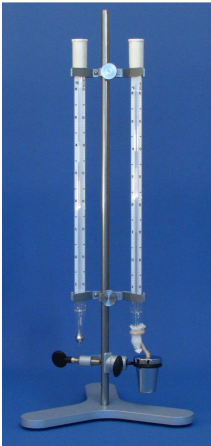
Fig.1 Psychrometer 28, August-Type, without ventilation, consisting of grey lacquered stand, with thermometer holders, water vessel with holder for 2 equal thermometers
