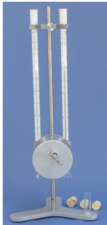
Fig. 2 Psychrometer 28/2 with large aspirator, for ventilation of both thermometers
